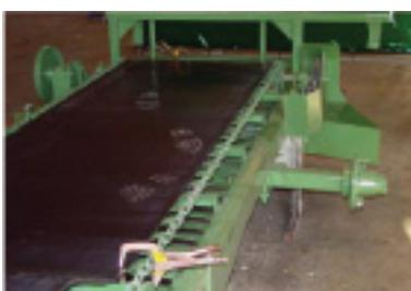
6. With the feed belt positioned square on the top side of the feedchain use a marker pen to mark where the tec screws are positioned depending upon the model of the feedchain. It is a good idea to use the old feedchain holes as a guide. However if you are replacing the **feedbelt only** use the alternative slats to avoid the existing holes in the feedchain.
