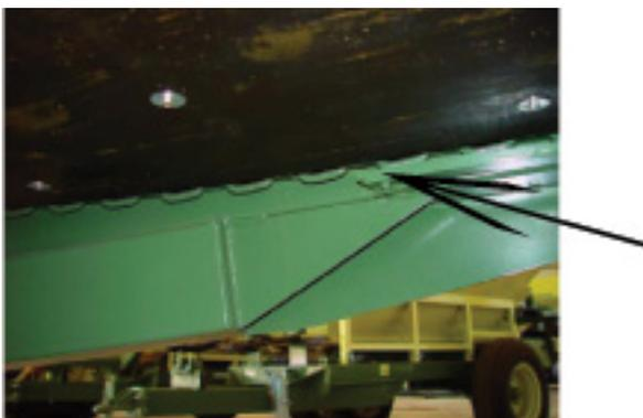
For 850T - 880T models tension chain to approximately 5mm above the front end of the nylon runner.
