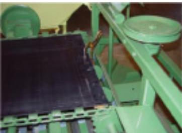
5. Also clamp the rubber to the feedchain at the front of the machine (As shown in the photo below).
