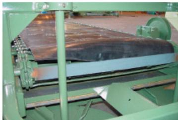
10. Once again clamp the section of the belt that will have the tecs now installed. Repeat steps 6-8.
