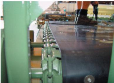
9. After installing the tec screws along the top side of the feedbelt unclamp the belt at the joiner slat and at the front of the machine. Turn the belt so that the section of the chain that has not had the rubber installed comes to the top of machine.
