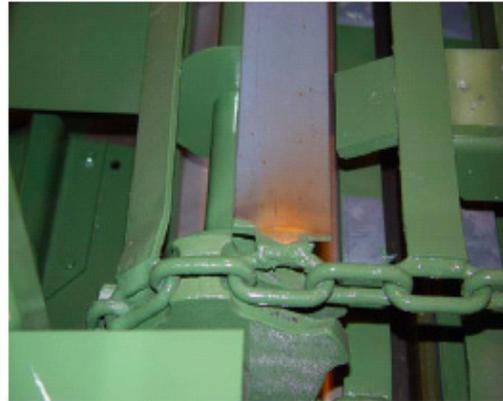
9. The next step is to tension the chain by using the two bolts located on the front idler shaft. Once the chain is tensioned ensure the slats are square by linking them up on top. The picture below shows the correct tensioning of the 825T and 840T models.
